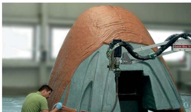
Design study about high speed train by means of **EP lay-up paste P 26**
