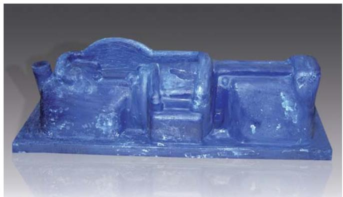
Blank for electroplating bath model dashboard of **ebablock**® P 185 blue
