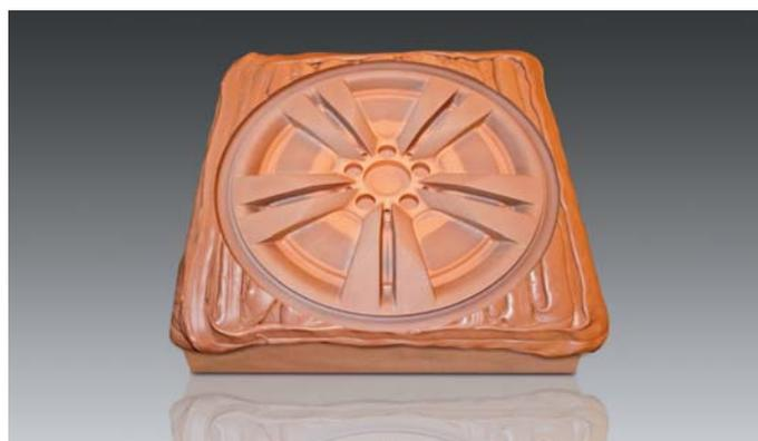
Base construction for car wheel rim made of **ebaboard L-1, EP lay-up paste P 26**
