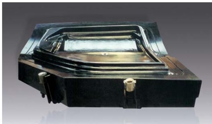
RTM mould of *ebalta* epoxy resin
