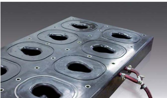
RTM mould with a surface of **OH 50**
