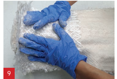
Press the A1 Triaxial fibre. The fibre can be formed/shaped well.
