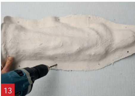
If needed, holes can be drilled in the A1 support mould to add bolts and nuts.
