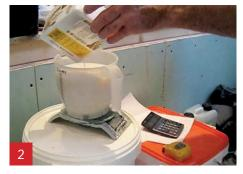
Weigh the correct amount of Component A (1 part in weight) and Component B (1.2 part in weight) + 2% colour pigment of your choice.
